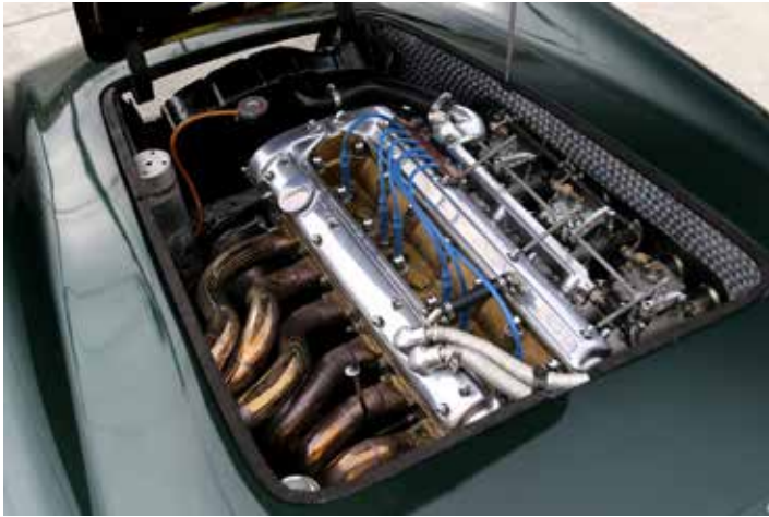
DOHC six cylinder upgraded to 400 hp
