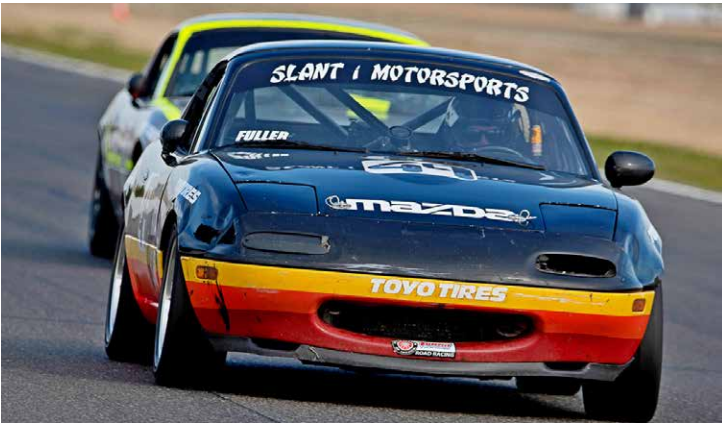
#49 Rob Fuller demonstrates that Spec Miata Racers will do anything for extra speed. Note the right side mirror tucked in on both cars.
