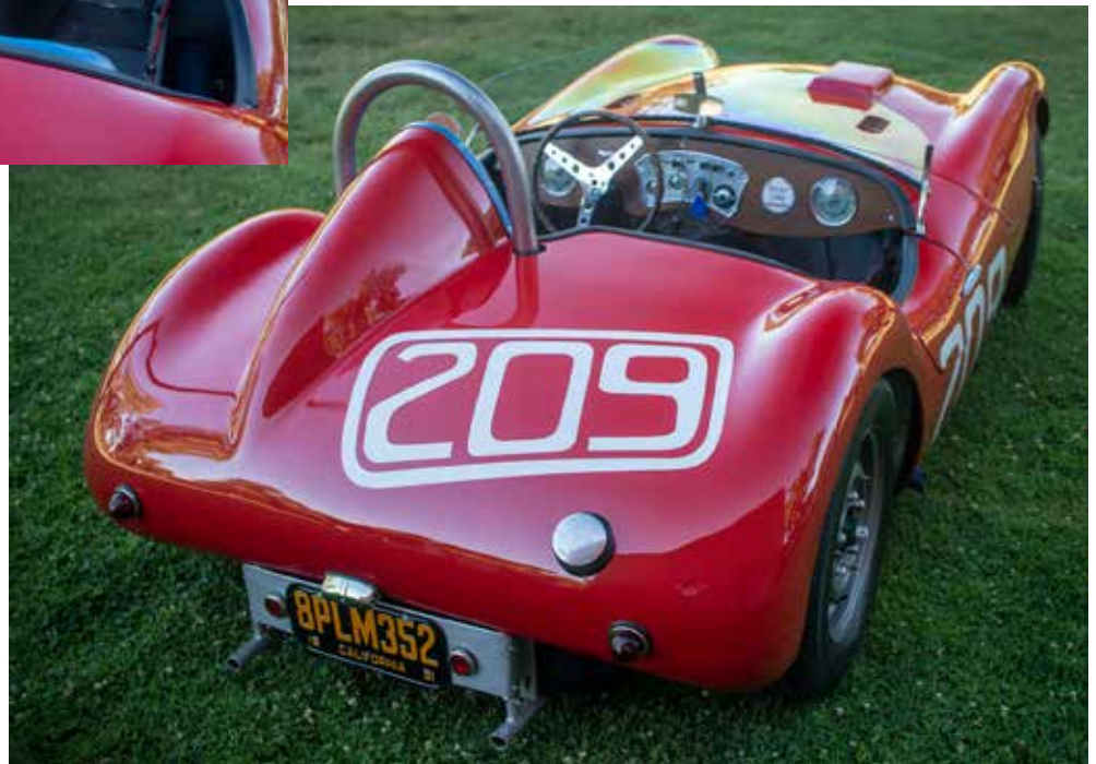
Ted designed and fabricated the fiberglass body, using his wife's Pyrex baking dish to mold the carburetor air scoop
