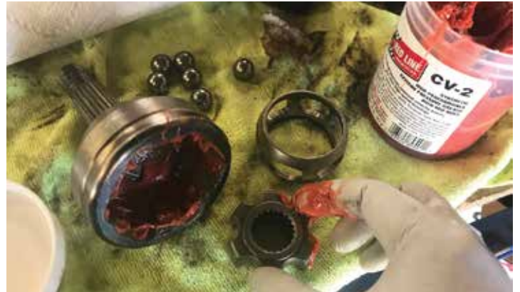
Halfshaft servicing reassemble with fresh grease
