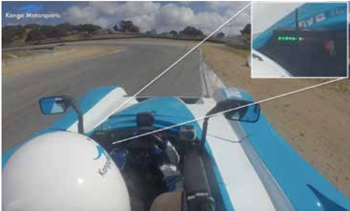
One Red light under braking going into Turn 5 indicates I can brake just a bit harder.
