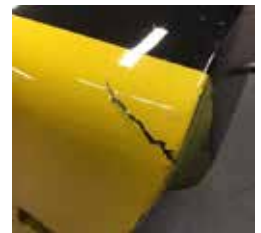
Typical Fiberglass Crack in Body
