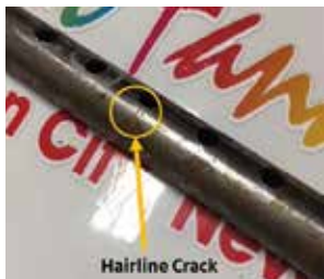
Example of a Crack in the Lower Tube
